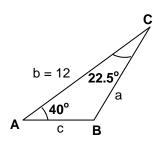
What if we are given 2 sides and an angle opposite only 1 of those sides (SSA)? This can result in different possibilities that can still be determined using the Law of Sines.
